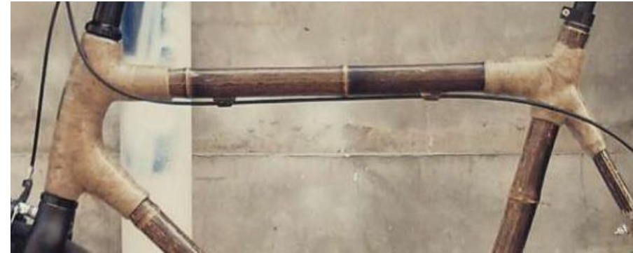
Hemp composite reinforcing the bamboo frame.
